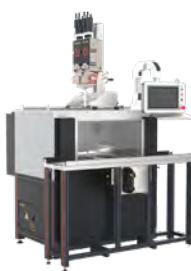
Vakuum chamber dos vac Vacuum chamber with integrated axis system for positioning components in 3 degrees of freedom.
