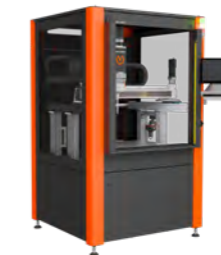
Stand-alone dos cell Axis system including protection cell for moving the dispenser through 3 degrees of freedom.
